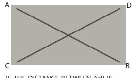
IF THE DISTANCE BETWEEN A-B IS EQUAL TO C-D, YOUR BASE IS SQUARE
